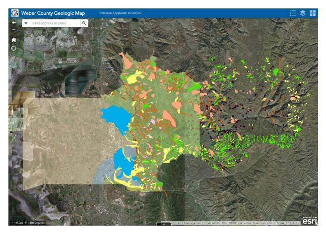
Shut off all of the layers except "parcels\_secure-Parcels", "Parcel Labels-Street Labels", "Engineering\_Layers-Wasatch Faults" and "Engineering\_Layers\_Geologic Faults" and then select the "Geologic-layers\_Ogden-shape\_ GeologicUnits" as shown below:
