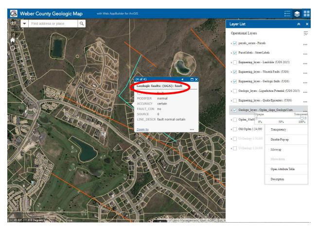
If the geologic unit associated with the parcel in question is identified in the list of units below or has a fault line identified on the site, a geologic site reconnaissance is required to determine if the building lot falls within a potential geologic hazard study area. If it is found that additional studies are necessary, a geologic and possibly a geotechnical analysis will be required if the engineering geologist hired by the applicant determines it necessary.
