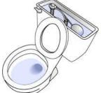
Put food coloring in the tank and if the color appears in the bowl without flushing there is a leak in your toilet.
