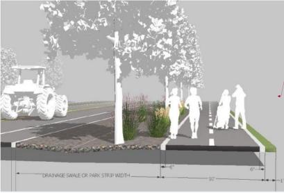
(3) Non-street-adjacent pathway. Where generally depicted on a map or in the text of an applicable street regulating plan, general plan, master streets plan, or when otherwise required herein or in a development agreement, a 10-foot wide hard-surfaced pathway shall be installed through the development.
