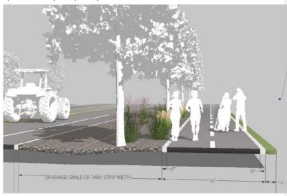
(3) Non-street-adjacent pathway. Where generally depicted on a map or in the text of an applicable street regulating plan, general plan, master streets plan, or when otherwise required herein or in a development agreement, a 10-foot wide hard-surfaced pathway shall be installed through the
