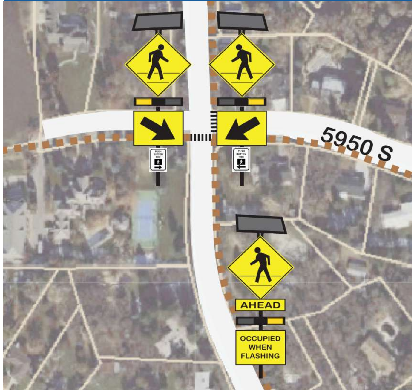
Map 16 - Pathway Street Crossing with Rapid Flashing LED Beacons
