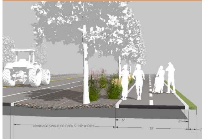
Figure 53 - Pathway Cross Section - Street Adjacent
